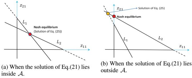
Fig. 3: Two cases of NE.  $x$  and  $y$  axes denote the request strategy of coalitions  $C_1$  and  $C_2$ , resp. The two lines  $L_1$  and  $L_2$  denote the *best responses curves* of coalitions  $C_1$  and  $C_2$  when the feasible region  $\mathcal{A}$  is relaxed, while the dashed line segments are outside the feasible region. Following Theorem 6, they are replaced by the dotted line segments.
